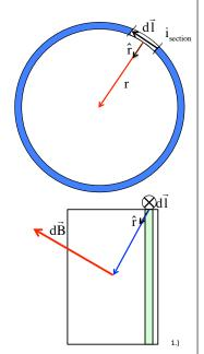
Look at the current section at the bottom of the swath. The vertical magnetic field components will add to zero leaving you with differential magnetic field pieces in the x-direction only. That means that the net field will be along the central axis of the hoop.
